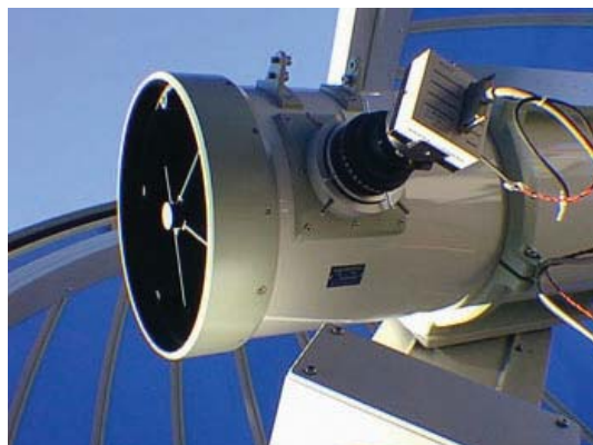
Fig.2 Optical telescope with 35-cm diameter (The square box in the upper right of the photograph is the cooled CCD camera.)
