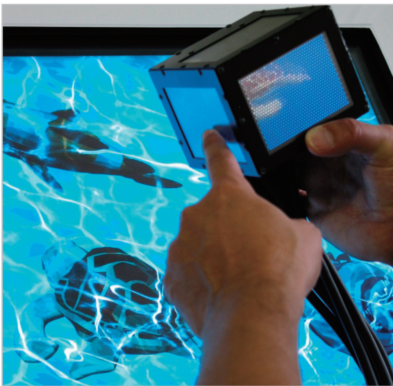
Fig.1 Interactive virtual 3D aquarium using the gCubik+i platform
