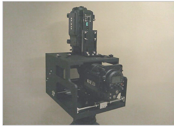
Fig.1 Ultra-high definition stereo 3D camera
