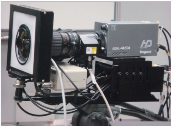
Fig.4 Rangefinder camera (Axi-Vision camera)
