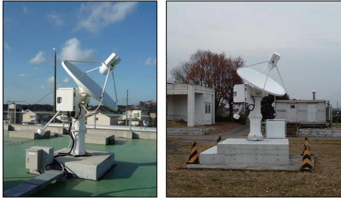
**Fig.9** Left: The first prototype of the MARBLE compact VLBI system at Kashima Space Technology Center, NICT. Right: The second prototype at the GSI, Tsukuba
