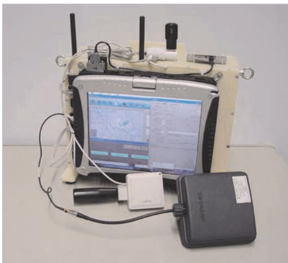
Fig. 142 Integrated multi-RFID reader/writer
