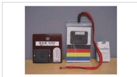
Fig.5 Hybrid tag attached to a damaged building (left), and triage tag attached to victim transported (right)
