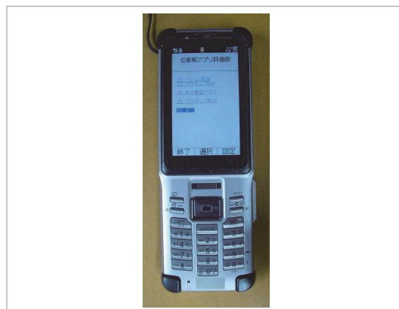
Fig. 130 Ubiquitous terminal containing UHF-band passive/active RFID reader/writer and the screen of message board application
