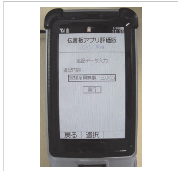
Fig. 141 Screen of a cell phone application that permits writing of message on passive RFID
