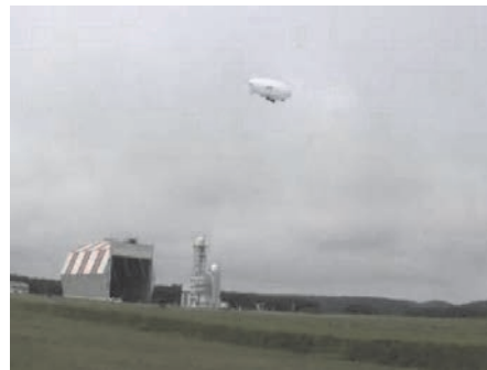
Fig.70 Test on collecting damage information from above by an unmanned airship
