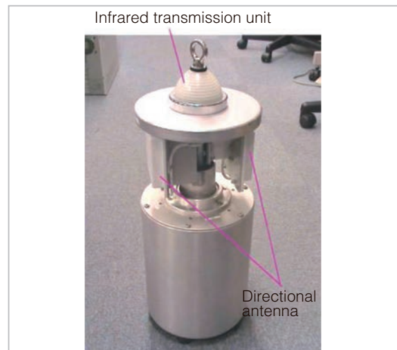
Fig.29 External appearance of the release-type pod communicator
