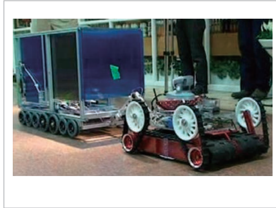
Fig. 17 Cable-laying system using a trailer
