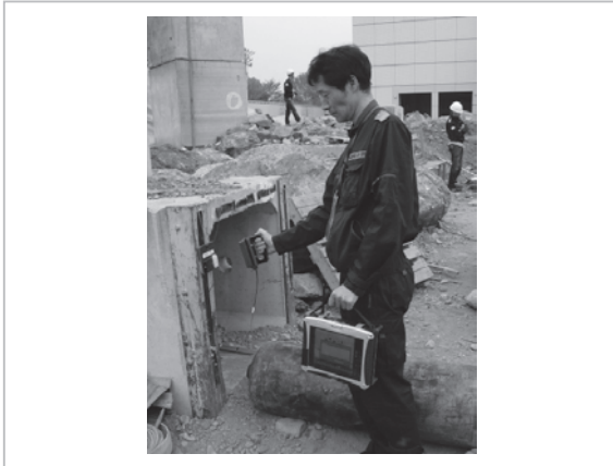
Fig.3 Usage of hybrid RFID reader-writer
