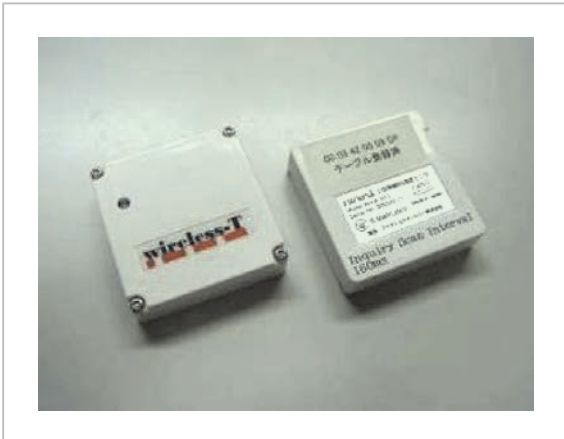
Fig. 12 Bluetooth device (small size wireless acceleration sensor) used instead of active RFID
