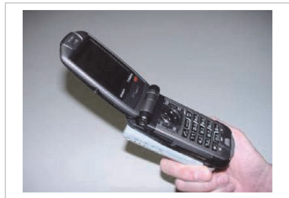
Fig. 11 Cell phone terminal equipped with passive RFID reader attachment (au E03CA)
