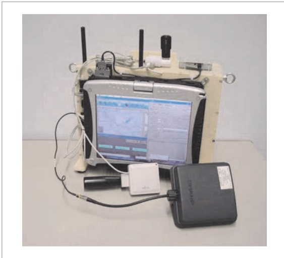
Fig.18 Prototype of integrated reader-writer with support for multiple RFIDs
