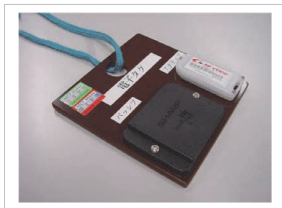
Fig.1 Hybrid RFID (left: passive RFID, right: active RFID)
