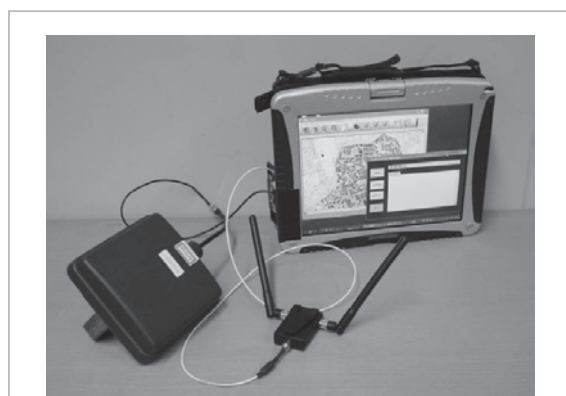
Fig.2 Hybrid RFID reader-writer (flat panel antenna is for passive RFID, diversity antenna is for active RFID)
