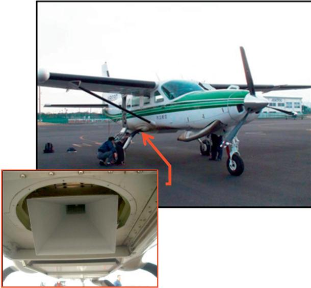
Fig. 4 Airplane (Cessna208B) and measuring horn antenna used for the measurement of the interference
