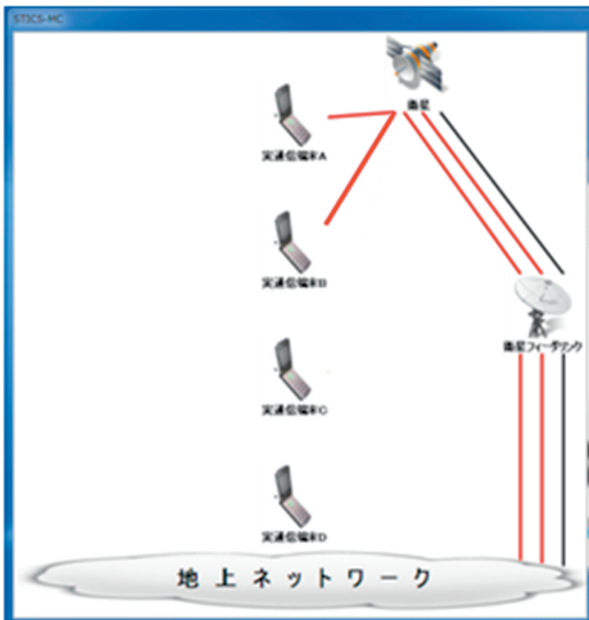
Fig. 29 Call at traffic congestion (Network dynamic resource control equipment) (Priority terminal)
