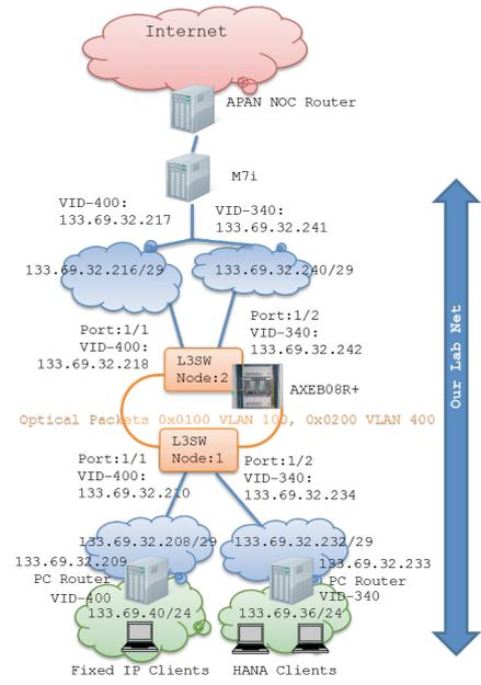
Fig. 8 Testbed enhancement by the use of optical packet switches having 12 10GbE interfaces
