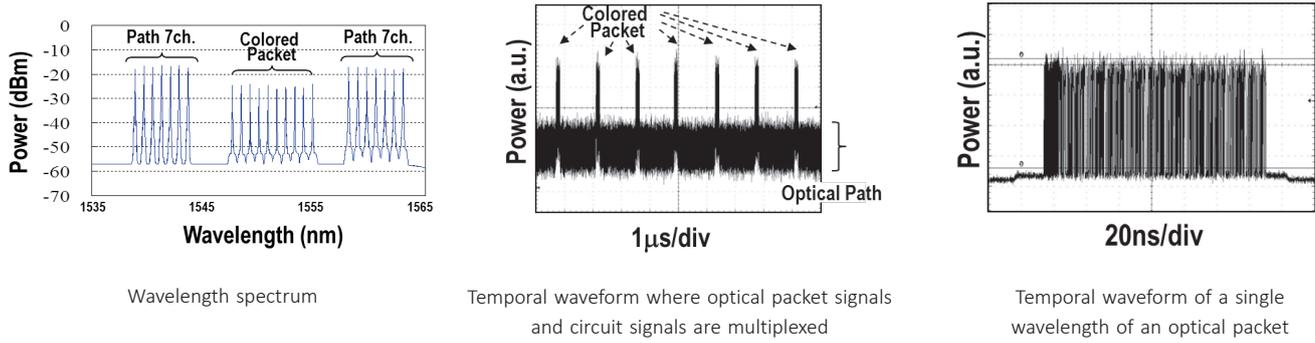
Fig. 5 Waveform of optical packet signals and circuit signals
