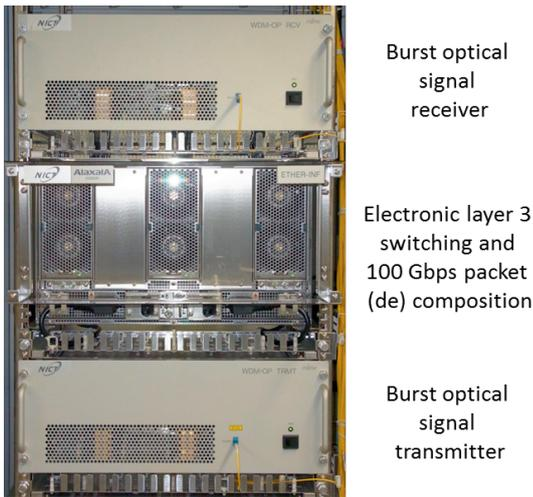
Fig. 9 A layer 3 switch capable of 100 Gbps optical packet interface and 12-port 10GbE
