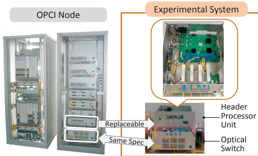
Fig. 13 Header processing unit for longest prefix matching address lookup and optical switch driven by the lookup result, which was been embedded in the OPCI node.
