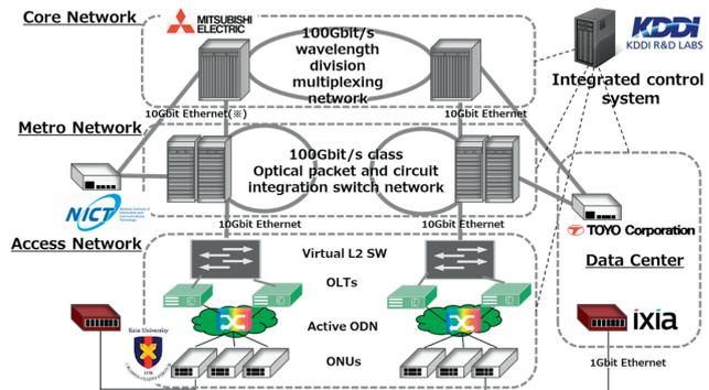
Fig. 11 An example optical transport network consisting of optical core, metro, and access networks and data centers integrated and managed by SDN (see NICT press<sup>[20]</sup>). It was demonstrated at iPOP 2014.
