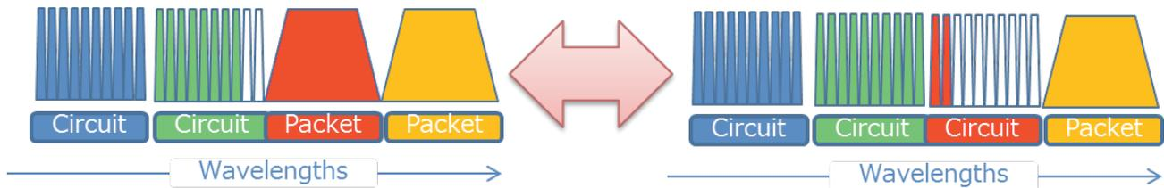
Fig. 6 Moving boundary between optical packet resources and optical circuit resources
