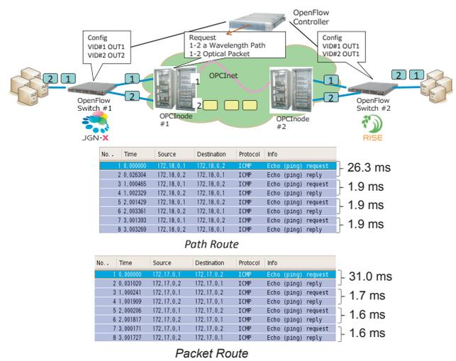
Fig. 10 A network consisting of RISE OpenFlow switches and OPCINodes and reachability check result. Delay for the first packet is longer than others, because a flow is added to the flow table at that time.
