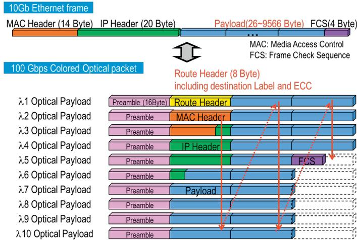
Fig. 3 Optical packet format
