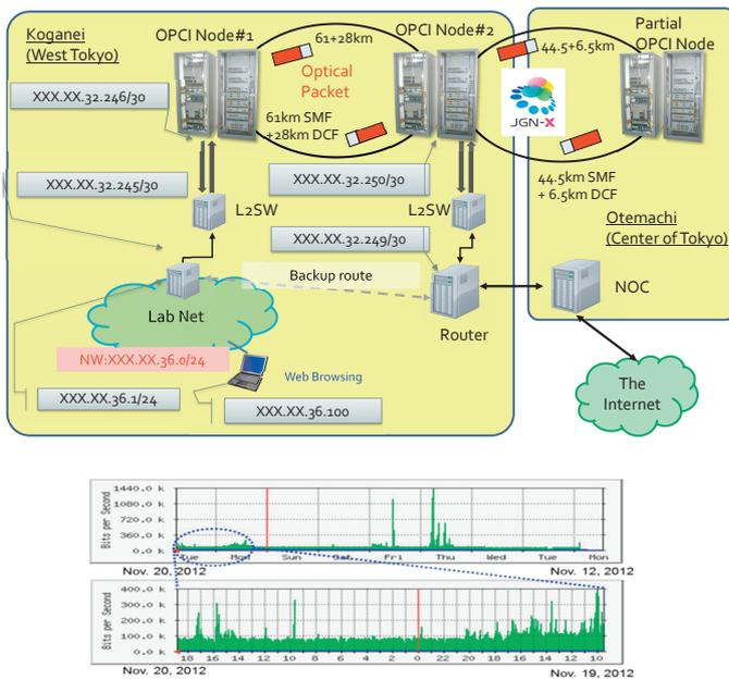
Fig. 7 OPCInet testbed by using laboratory network and JGN-X
