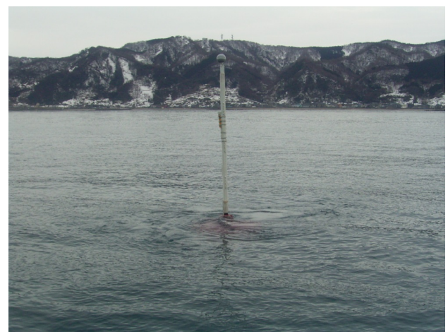
Fig. 4 Fixed target at 1 NM from the radar (a spar buoy)
