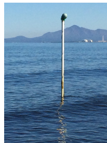
Fig. 3 Target installed at 40 m from the radar
