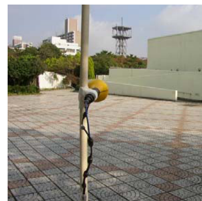
Fig. 11 Schematic showing the measurement of electric field strength around the base station using the electric field probe
