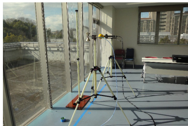
Fig. 21 Small probe for measuring tri-axial isotropic electric fields (rear) and broadband antenna (front)
