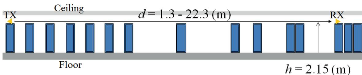
Fig. 10 Positions of metallic server (Copyright(C)2017 IEICE, [4] Fig. 2)
