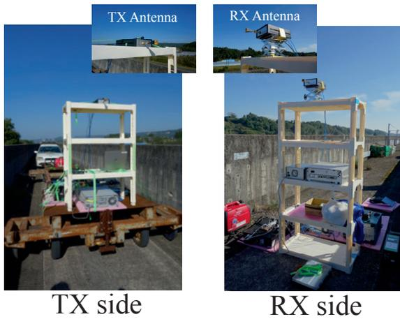
Fig. 1 Propagation measurement in viaduct environment (Copyright(C)2017 IEICE, [2] Fig. 4)
