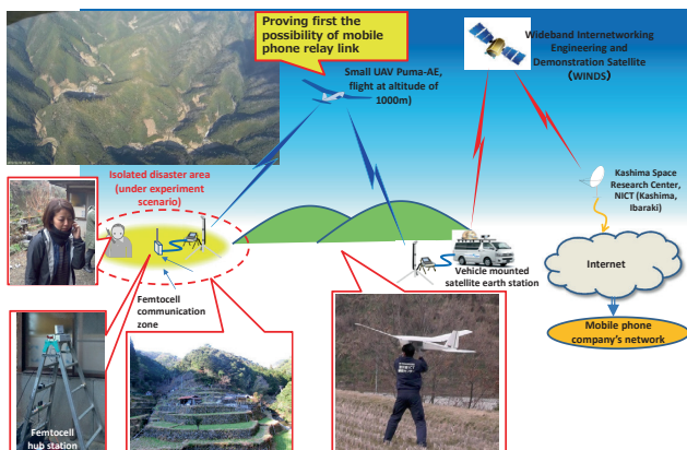
Fig. 6 Experiment of mobile phone link by air to space relay (Shimanto-cho, Kochi, February 2015)
