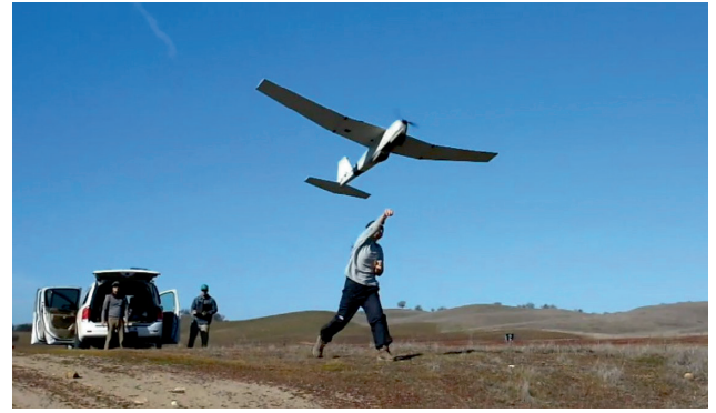
Fig. 3 Throwing launch of communication-link drone
