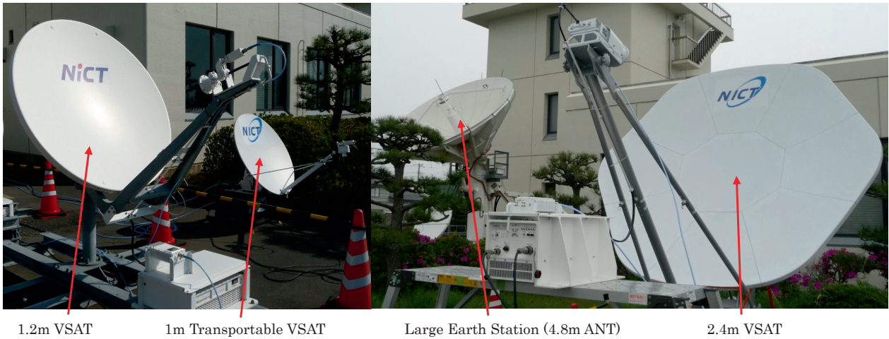
Fig. 1 Outdoor equipment for experiment of regenerative link rain attenuation compensation
