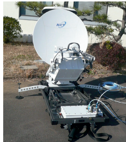
Fig. 2 Fully automatic earth station
