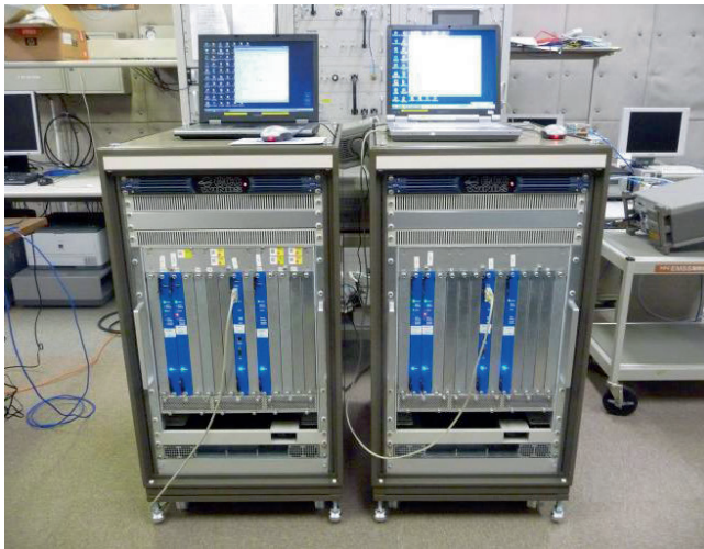
Fig. 7 622/1244 Mbps Dual-Rate Burst Modems (two sets)
