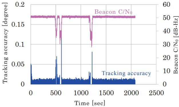
Fig. 11 Tracking accuracy at cruise of figure eight
