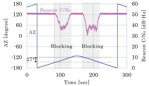
Fig. 8 Verification of communication blocking area
