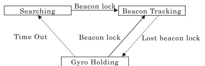
Fig. 3 Process of acquisition and tracking
