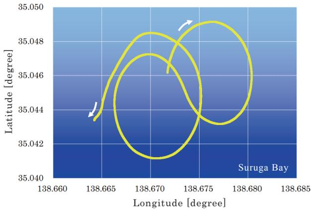
Fig. 6 Trajectory of figure eight cruise
