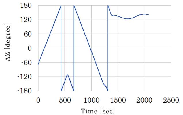
Fig. 9 The angle of azimuth motion situation of the antenna at cruise of figure eight
