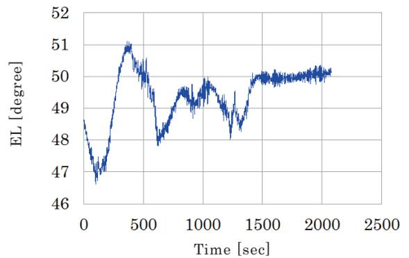
Fig. 10 The angle of elevation motion situation of the antenna at cruise of figure eight
