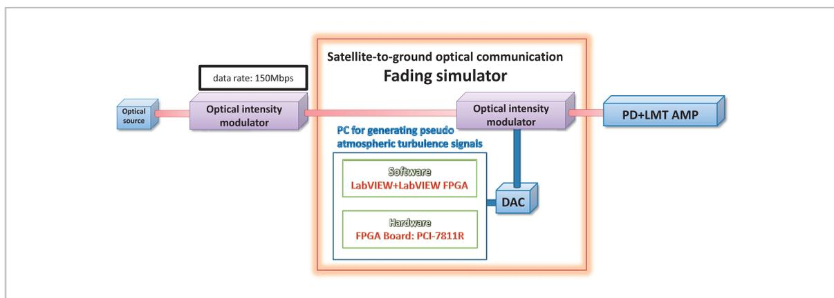
**Fig.8** Configuration of the communication experiment system using the simulator
