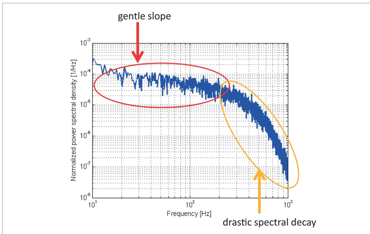
**Fig.5** Results of Fourier transformed waveforms of optical signals under atmospheric turbulence measured at OICETS experiment
