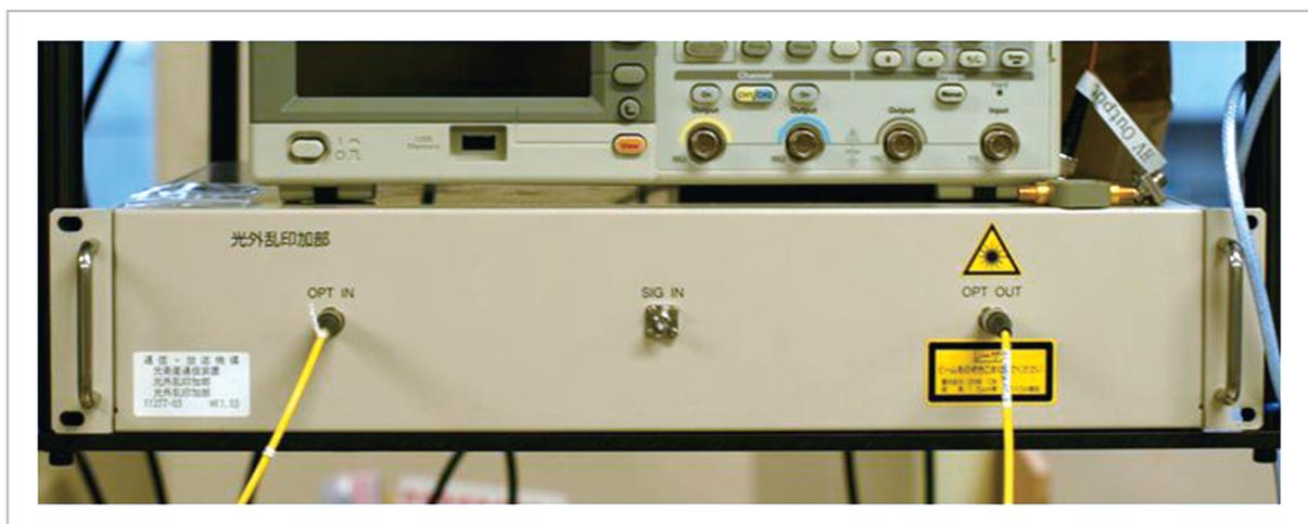
**Fig.2** Optical intensity modulator
