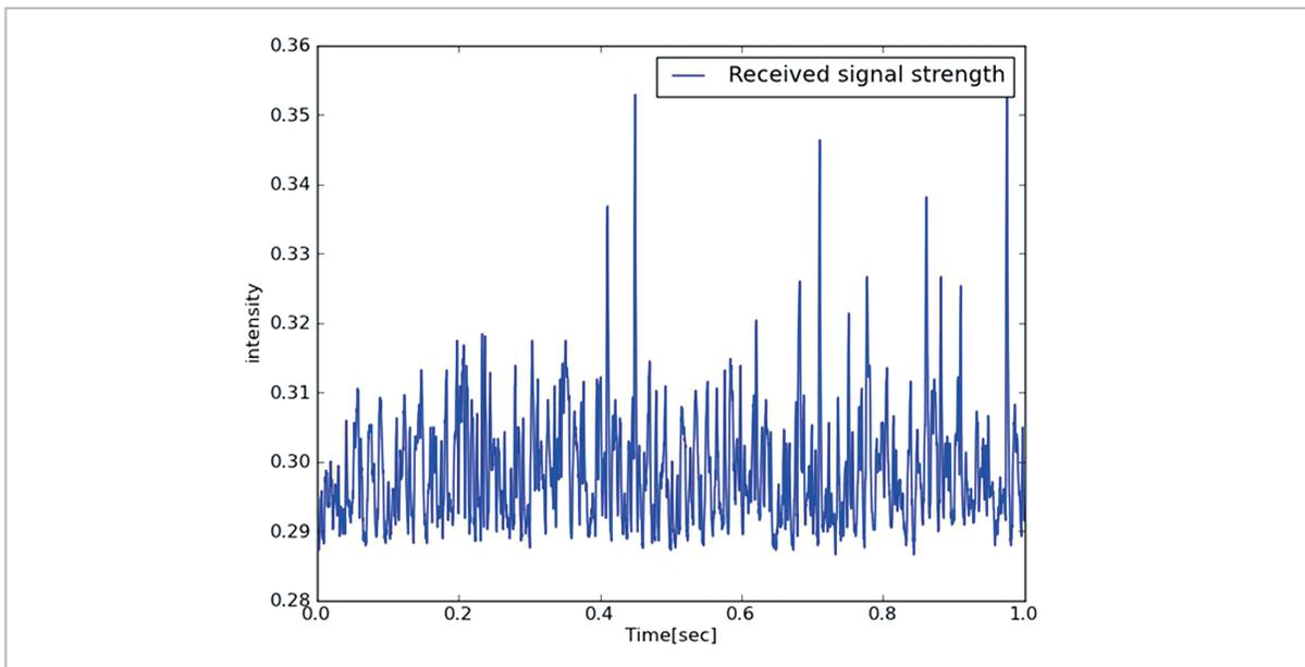
**Fig.6** Variations in the received signal level caused by pseudo atmospheric turbulence generated in the optical fiber
