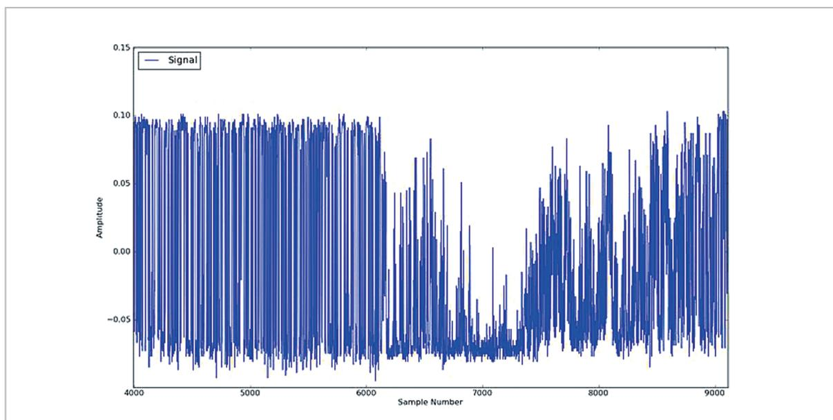
**Fig.9** Received signal level propagated through pseudo atmospheric turbulence
