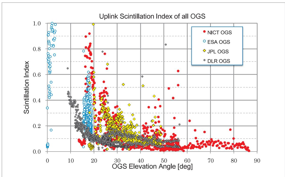
**Fig.2** Relationship between scintillation index and elevation angle at each ground station
