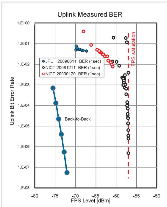
**Fig.8** BER characteristics obtained in NICT and JPL experiments
