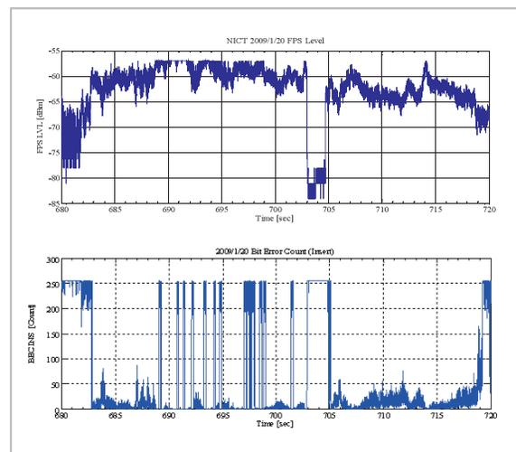
**Fig.7** FPS received signal level and number of insertion errors in experiments with NICT station
