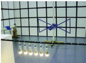
電波暗室と反射箱におけるLED照明から放射される電磁雑音の測定風景 Measurement of EM noise radiated from LED lighting in anechoic and reverberation chambers
