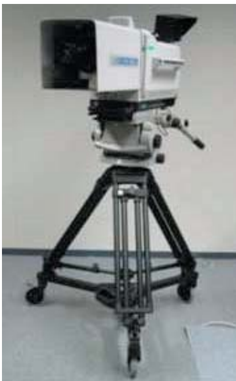
Figure 3: Super-high-definition (8 million pixels) CMOS Video Camera
