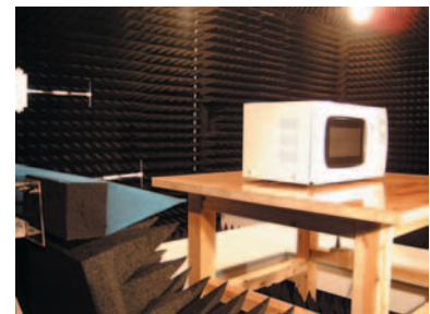
Figure 4: Centers of Wave Emissions Estimated from Measurement of Leakage Waves from Microwave Oven
