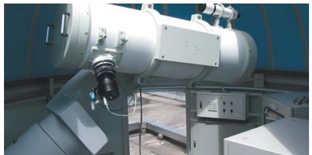
Figure 2: Optical observation system for geostationary satellites
