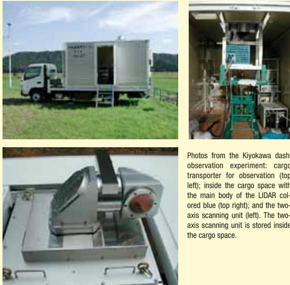
Photos from the Kiyokawa dashi observation experiment: cargo transporter for observation (top left); inside the cargo space with the main body of the LIDAR colored blue (top right); and the two-axis scanning unit (left). The two-axis scanning unit is stored inside the cargo space.
