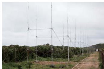
Figure 1 ● Receiving antenna for the long range ocean radar
