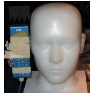
Photo 2: Appearance of the measurement of SAR using a human head phantom
