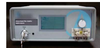
Low distortion optical amplifier for burst-mode optical signal
