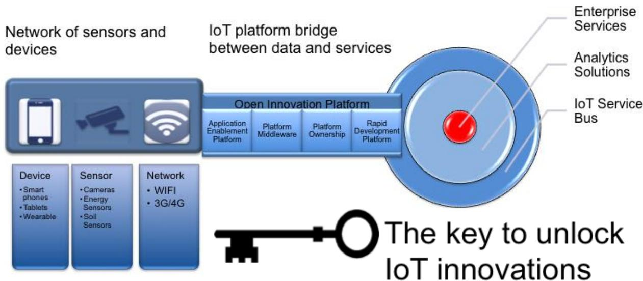
**Application enablement platform** provides abstraction layer to connect to the different devices available. Application dashboard tool to generate information visualization via easy to use interface.
