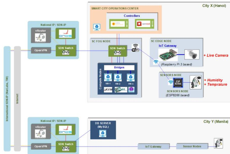
Diagram 3: Experimental Testbed Setup (source and acknowledgement: VNU)
