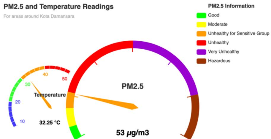
Diagram 1: A Simple Web based dashboard for Air Quality Sensor (source: MIMOS)
