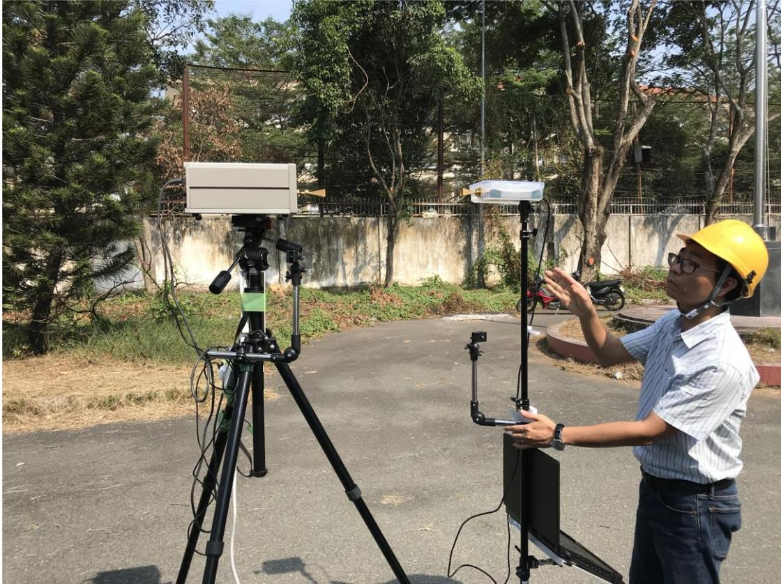
**Figure 26 Receiver with Anritsu MS2760A-0110**
