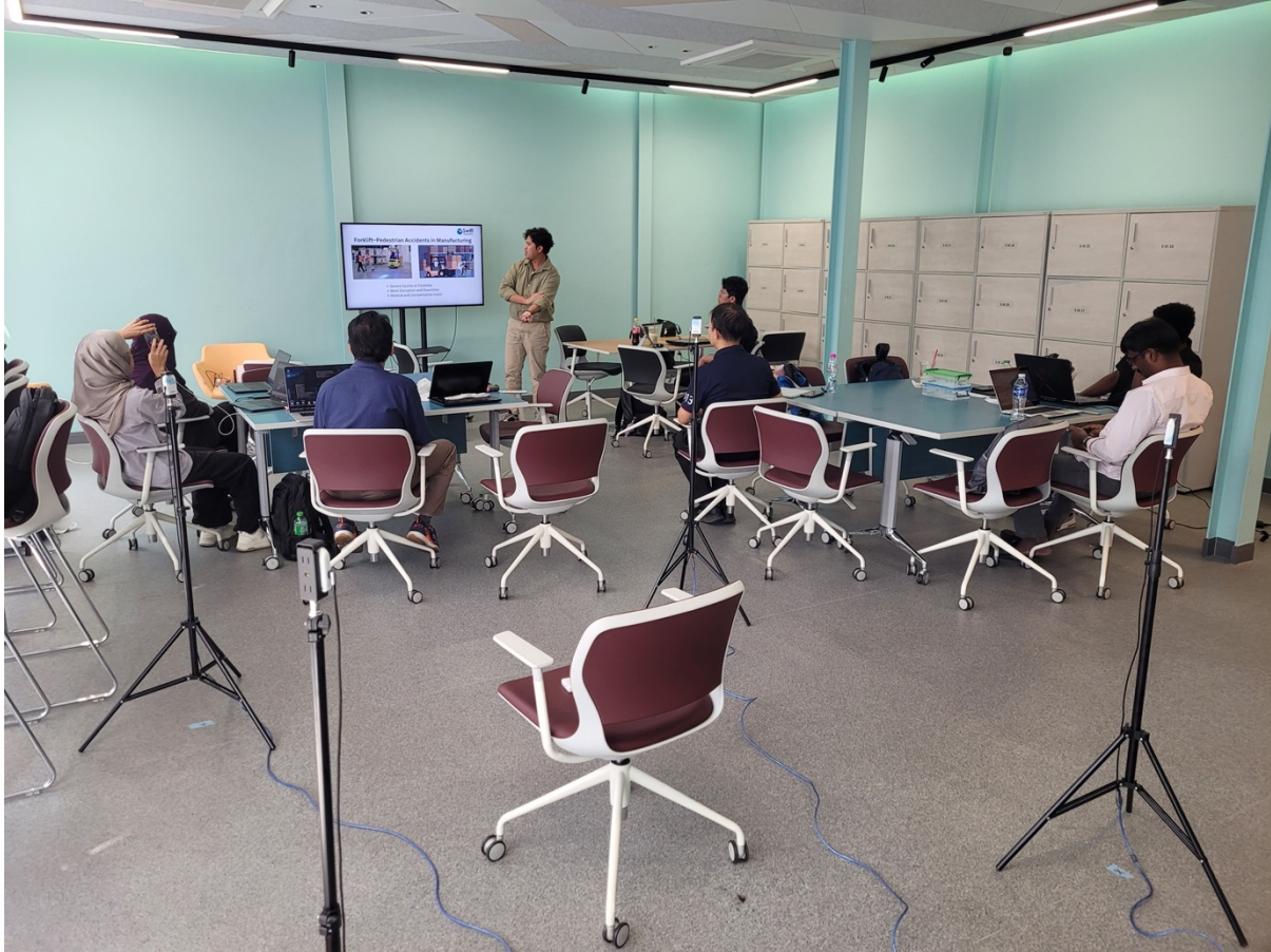
Setup of UWB infrastructure with 4 anchors
