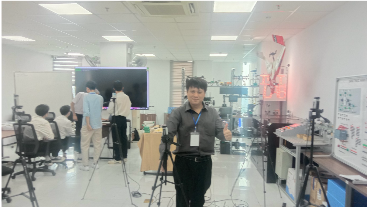
Setup of UWB infrastructure with 4 anchors with an active UWB tag within coverage
