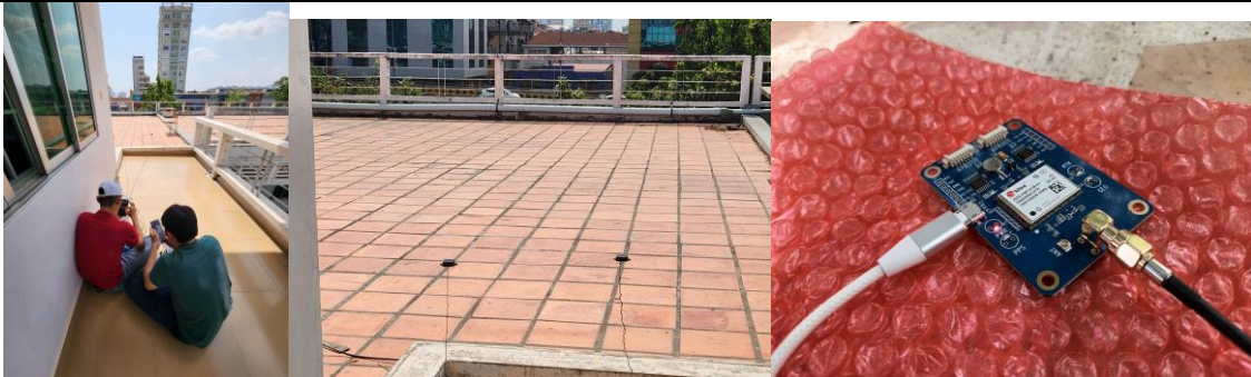
Fig. 17. Testing low-cost RTK receiver system using the new ITC and existing CADT stations as base stations on the first day. (Dr. Sophan, and Dr. Phimmasone).
