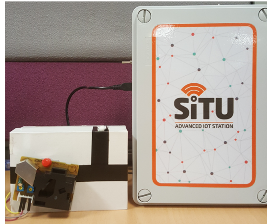
Figure 42 Completed sensor node with the hybrid IoT gateway developed by the project team
