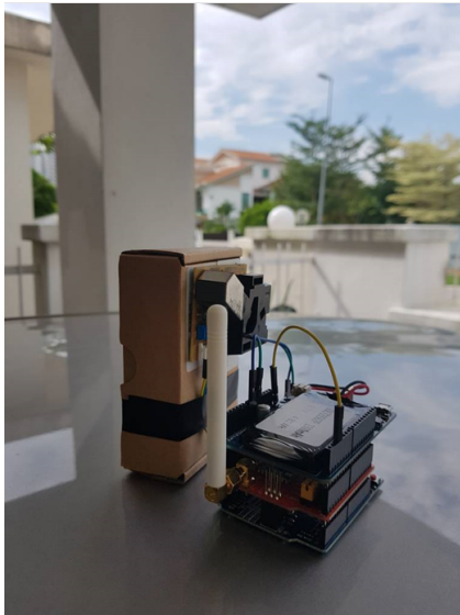
Figure 42 Completed sensor node with the hybrid IoT gateway developed by the project team
