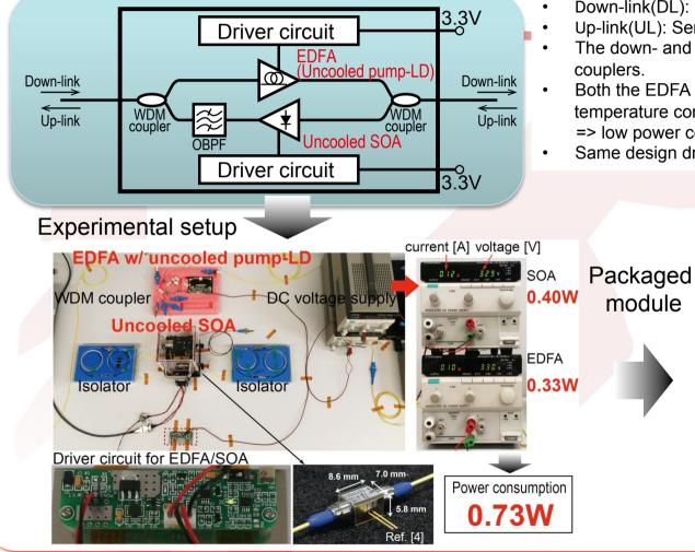
The power consumption is as low as 0.73-W in total ! The devices can be packaged in MSA-size module.
