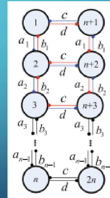
Topological structures with six coupled Hopf oscillators: a two-way double chain
