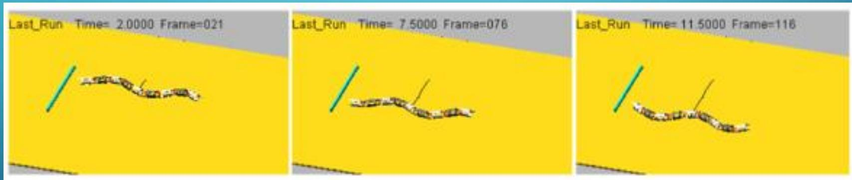
The screenshots of the simulated snake robot during the sidewinding gait on ADAMS. Main parameters are  $\omega = 1\text{Hz}$ ,  $\rho = p/6\text{rad}$ ,  $\rho R = p/36\text{ rad}$ ,  $\varphi = p/2\text{rad}$ ,  $d = 3p/10\text{ rad}$
