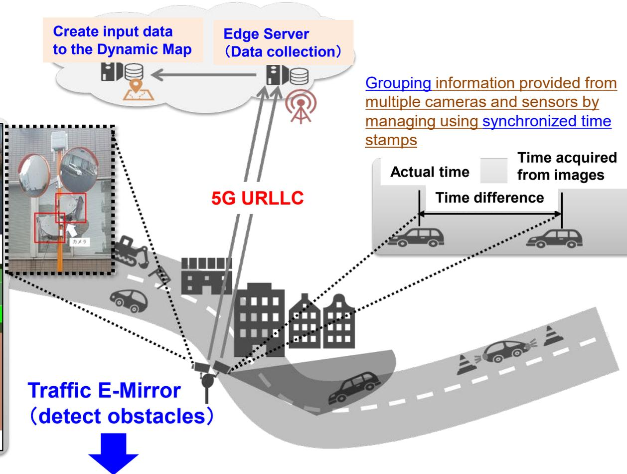
Grouping information provided from multiple cameras and sensors by managing using synchronized time stamps
