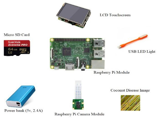
The camera will capture the coconut leaf or stem, with the captured image being sent to the Raspberry Pi module where the processing will be done. It will then be compared to the stored data of the neural network in the micro storage device. The Asus power bank will serve as the power supply with 2.4 Amperes meeting the required current needed to power up the Raspberry Pi module. An LCD touchscreen will be used as the output to show the classification of the image presented.
