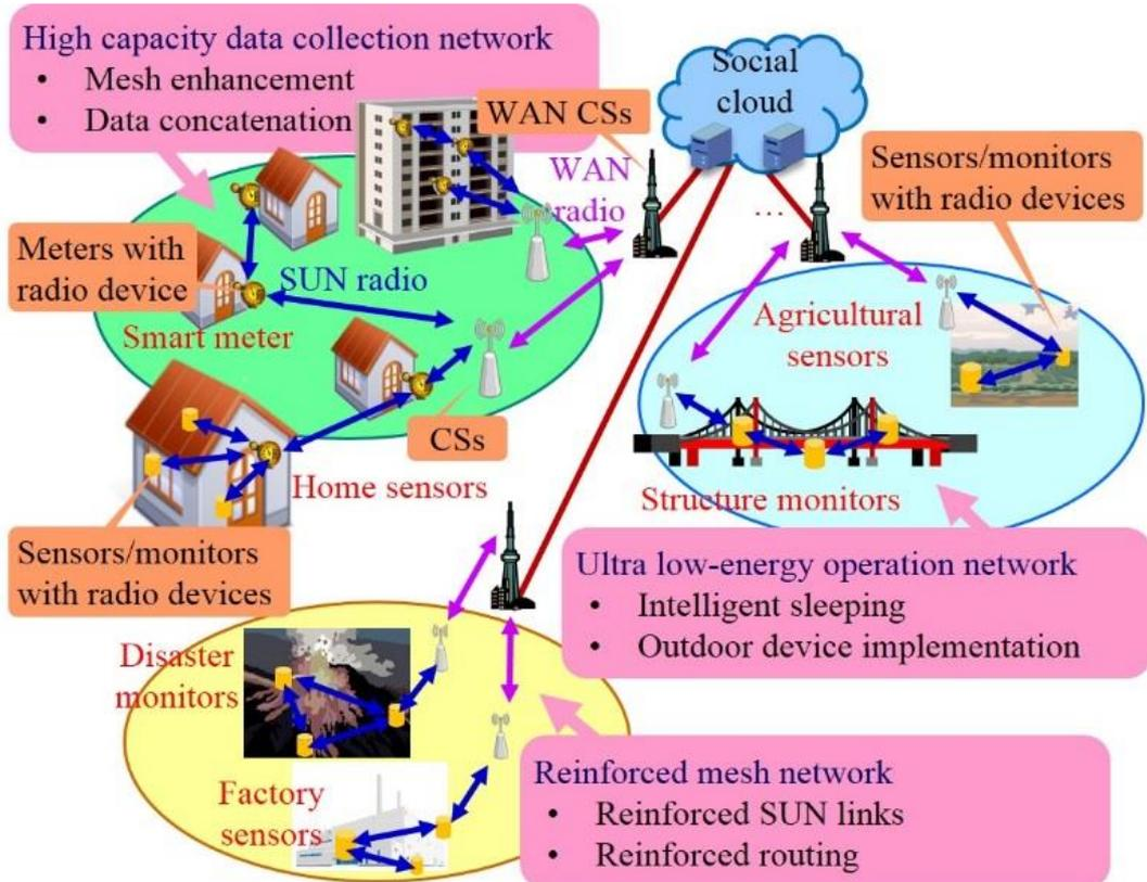
Fundamental categories for assumed wireless grid system exploiting SUN systems
