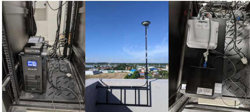
Fig. 2. GNSS receiver system equipment at CADT, Cambodia after setup.
