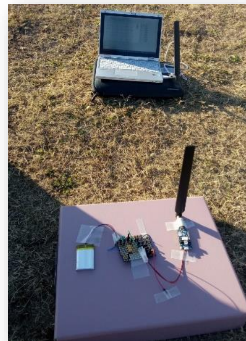
Field tested in Chofu-shi, Tokyo, Japan - Maximum range: 600 m
