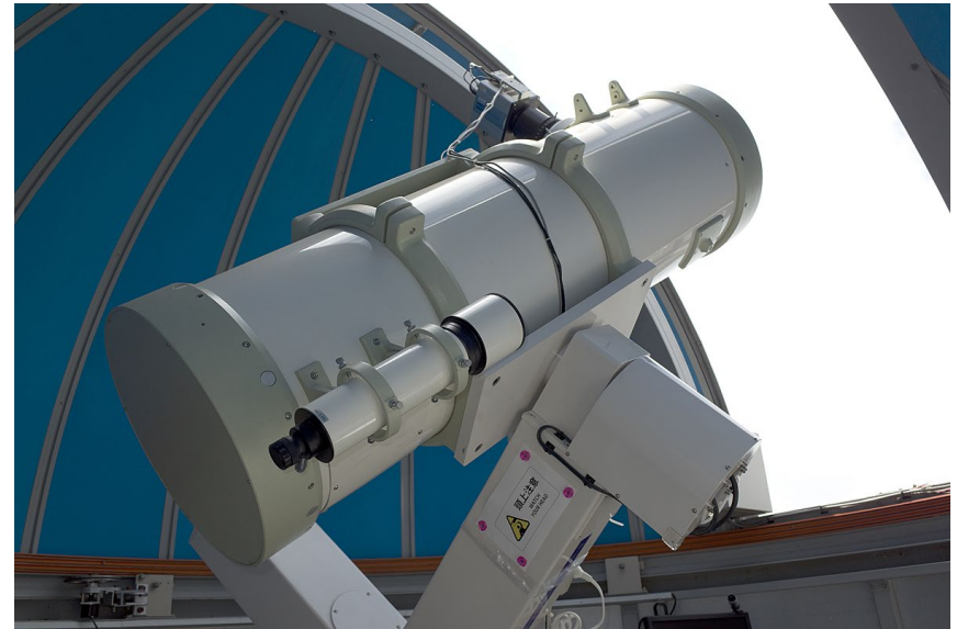
Kashima 35 cm telescope for satellite observation
