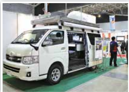
In-vehicle small mobile station for WINDS
