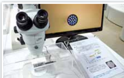
19-core optical fiber only observable via microscope
