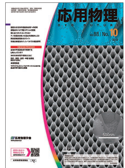
Figure 2 Cover of the October 2019 issue of the Japanese Journal of Applied Physics showing a scanning electron microscope (SEM) picture of the nanophotonic structure formed on the developed DUV-LED, with the author's comments
