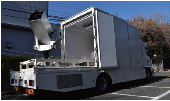
Figure 2 Portable optical ground station that stably receives the quantum signal from a satellite and can be deployed to various places
