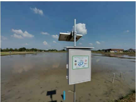
Figure Field trial of a water management system for paddy fields using IoT technology (Chiang Mai area, Thailand)
