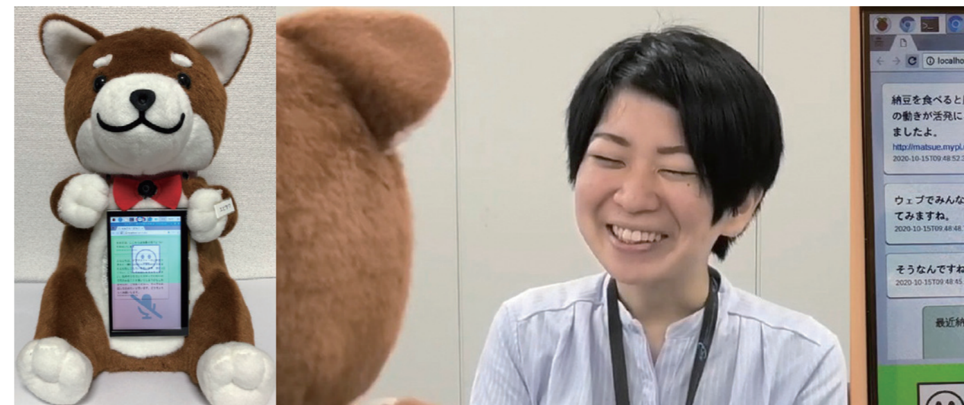
Figure Shiba inu dog-like MICSUS device engaging in conversation with a person (an NICT engineer). Dialogue records are displayed on the device's display (right). This technology was developed jointly by NICT, KDDI Corporation, NEC Solution Innovators, Ltd. and the Japan Research Institute, Ltd. with the support of the Cabinet Office's Cross-ministerial Strategic Innovation Promotion Program (SIP).
