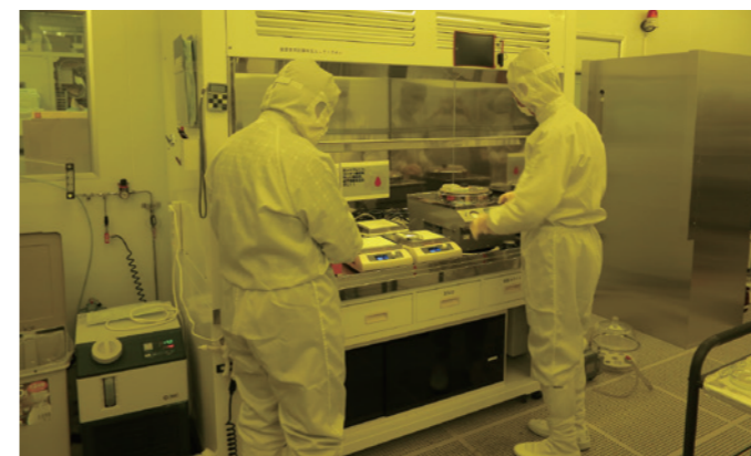
Figure 1 A scene with staff working in the yellow room (photoresist coating work)
