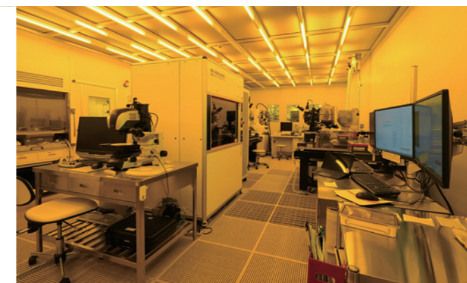
Figure 2 Inside the yellow room at the Advanced ICT Device Laboratory (Lithography equipment capable of nano/micro-sized photolithography)
