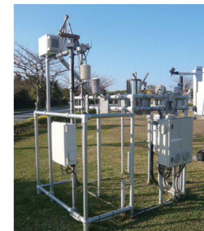
Figure 3 Exterior of environmental data collection device (Okinawa)
